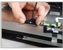
Before completely separating the screen from the rear casing you will carefully detach two wires that are connected to both sides of the device. This will allow you to completely separate the rear casing from screen.
