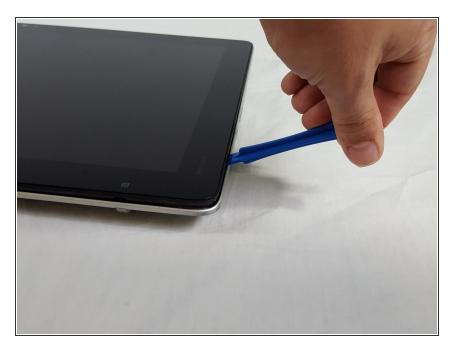
Using the plastic opening tool, carefully pry around the perimeter of the screen until the entire screen is completely separated from the rear casing.
