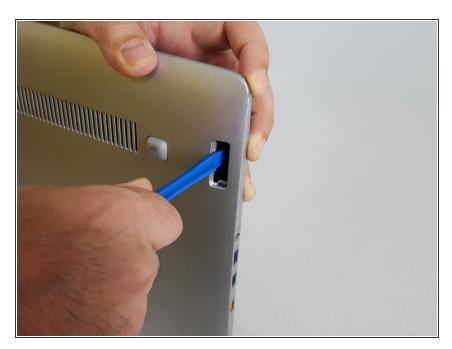
Using the plastic opening tool, push the display screen on the device forward until it separates from the rear casing.
