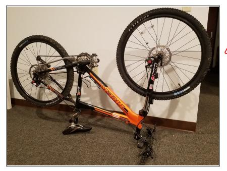
• Carefully flip bike over, balancing it on the handle bars and seat.
