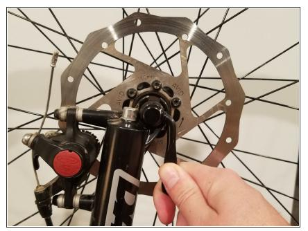
Release the clamping mechanism that holds the front forks to the wheel bearing by twisting it 180 degrees.
