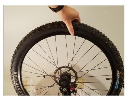
• Remove the front wheel from the forks by lifting it straight up.
