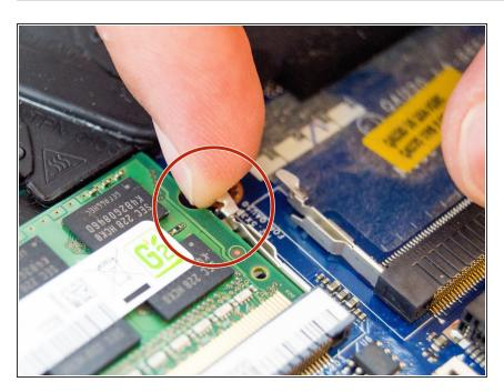
Pull the two metal tabs on the left and right sides away from the chip.
