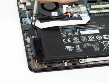
• Use the Philips #0 screwdriver to remove the three 4.2mm screws that are securing the battery to the board.
