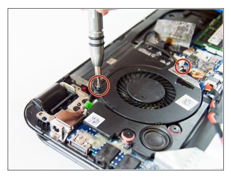
Using the Phillips #0 screwdriver unscrew the two 4.2mm screws fastening the CPU fan to the heatsink and motherboard.
