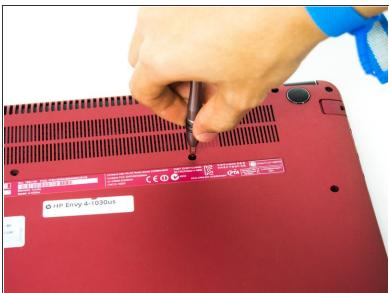
Using the Philips #0 screwdriver, remove the 12 7.5mm screws from the bottom cover.
