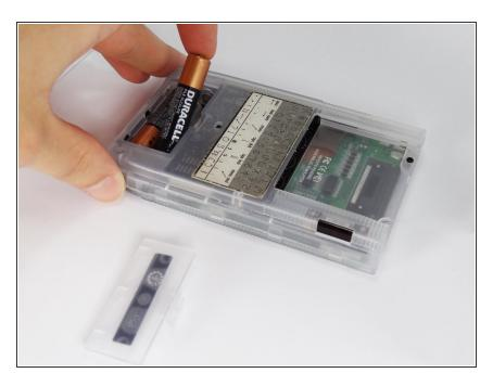
Remove the batteries from the device.
