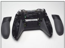
⚠ Be careful not to break the plastic tabs, that hold each grip cover to the back of the controller.
