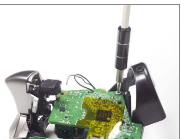
• Use the T6 Torx screwdriver to remove the two T6 7mm screws located just above the rumble motor housing.
