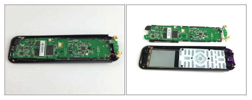
• Pull the circuit board off of the remote from the bottom, and lift up to detach it from the cover.
