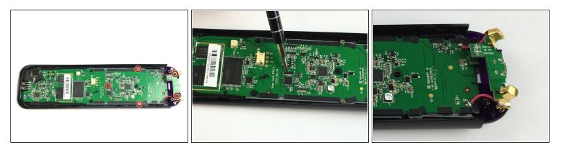
• Use the Phillips #0 screwdriver to remove the (5) five 6mm screws.
