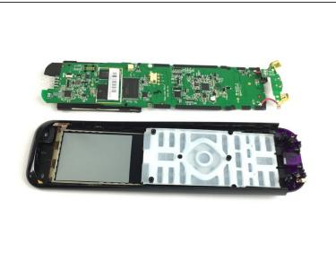
Pull the circuit board off of the case. Start from the bottom, and lift up to completely detach it from the cover.
