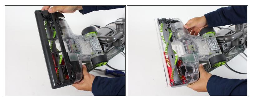
• Lift the plate up and off the vacuum head.
