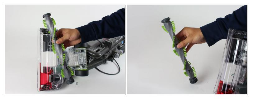
• Pull the brush roll away from the belt and remove the old brush roll.
