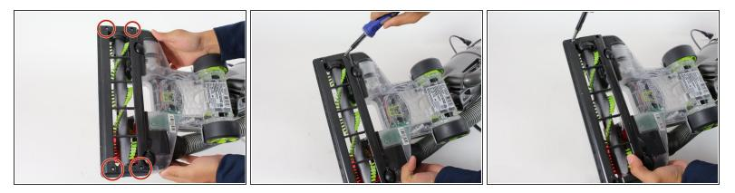
• Remove the 4 phillips 3/4" screws that hold the bottom plate.
