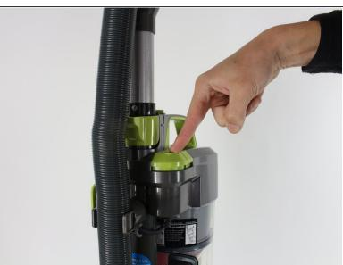
Put the cleaner into the upright position, turn the power off, and unplug the power cord.
