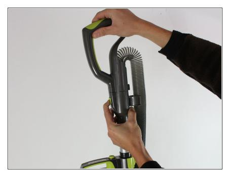
Press firmly on the hose button and slide hose out.
