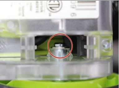
Locate the small metal pin and bolt holding the wheel in place.
