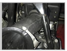
Using a 3/8"(9.525 mm) socket on the 3/8" ratchet, remove the air horn bolts, and pull the air horn out.
