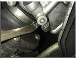
Using a flat head screw driver, loosen the hose clamps on the carburetor boots so that it can be removed later.
