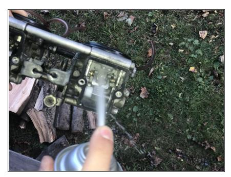
Spray the carb cleaner on the top part of the carb. Ensure clean mechanical action of needle guide.
