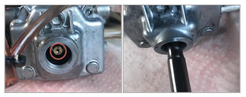
Remove the main jet with a 1/4" deep socket on a 1/4" ratchet.
