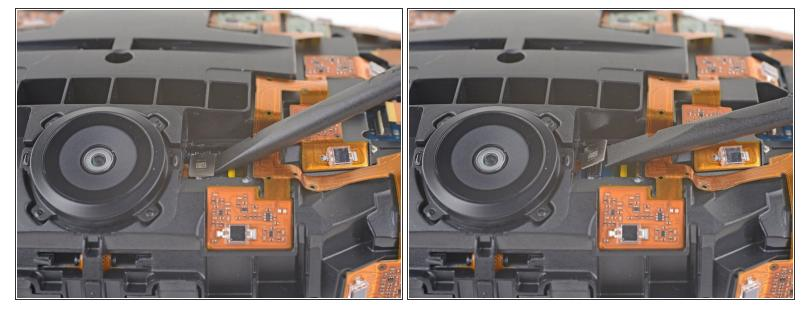
Use the flat end of a spudger to pry the camera cable connector straight up from its socket on the motherboard.
