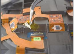
Use tweezers to remove the clear tape over all four of the sensor array cable connectors.
