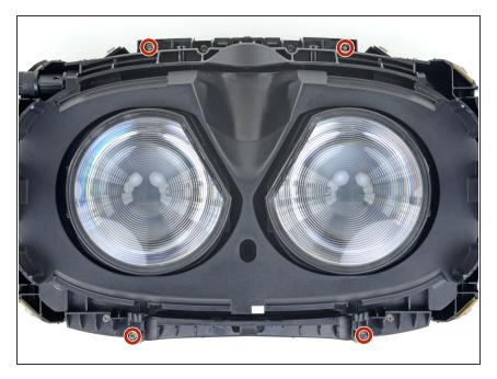
Use a PH000 driver to remove the four 3.9 mm screws securing the sensor array.
