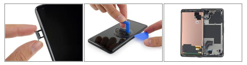
• Waterproofing a smartphone means sealing up all of the ingress points. We find our first evidence of Google's efforts in a gasket on the SIM tray.
