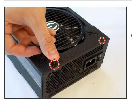
Using the 2mm Hex Key, remove the four screws located on the four corners on the bottom (fan side) of the power supply.
