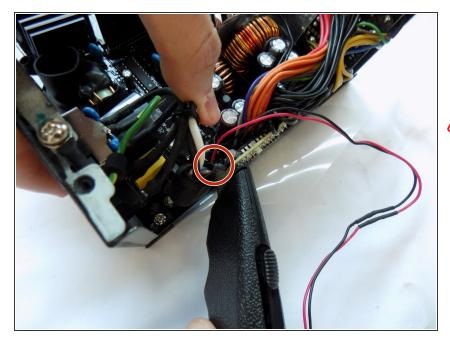
Cut the gray welding caulk material so that you can remove the fan from the motherboard
