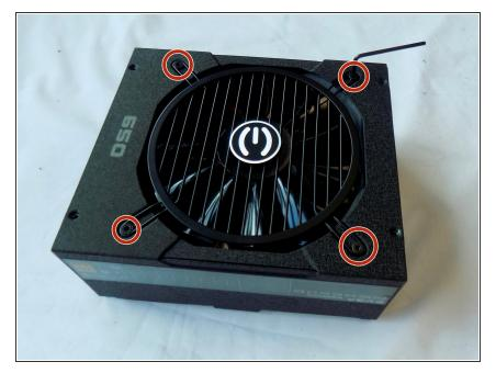
• Using the 2.5 mm Hex Key, remove the four screws holding the fan and its vent on the power supply.
