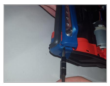
On the top side of the vacuum head, where the LED is located, use the Small Flathead screwdriver to pry open the cover. There should be no resistance.
