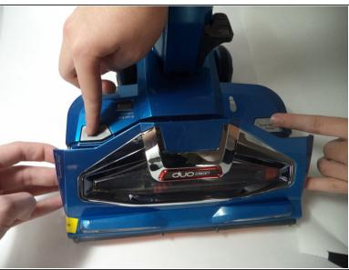
• On the top of the vacuum head is two grey "Brush Roller Access" buttons. Simultaneously press both buttons to eject the Roller Cover. Remove the Roller Cover by pulling it towards you and up.
