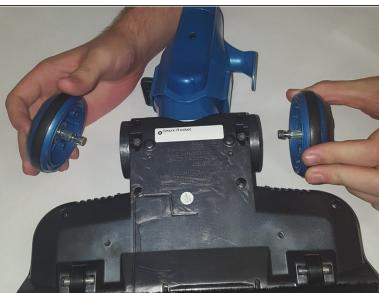
On the back of the vacuum head, locate and unscrew the four T15 screws. Once done the wheels can be removed.
