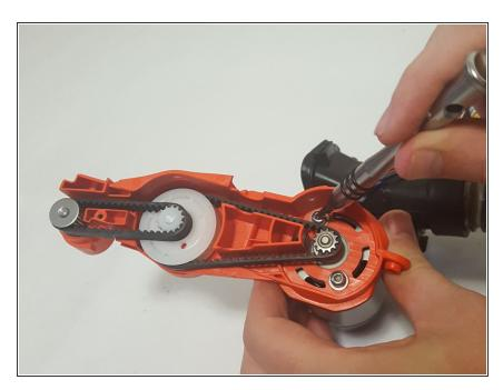
You now have access to the engine! This step is entirely optional, but the orange rotary piece can be removed using the T10 Screwdriver on the screws shown here.
