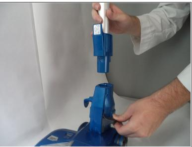
On the right-bottom of the body, pull down the black switch. You will hear an audible click when you detach the body from the vacuum head.
