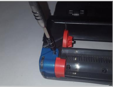
On the back of the vacuum head, located near the bottom, should be a row of screws. Using the T15 Screwdriver, remove all the screws on the bottom and the sides.
