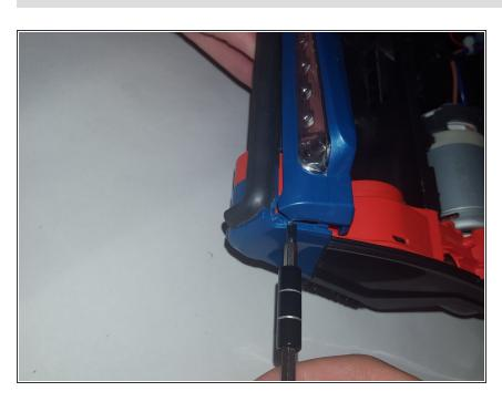
On the top side of the vacuum head, where the LED is located, use the Small Flathead screwdriver to pry open the cover. There should be no resistance.
