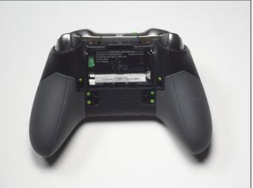
Remove the two batteries AA batteries by lifting them from one end and pulling them out.
