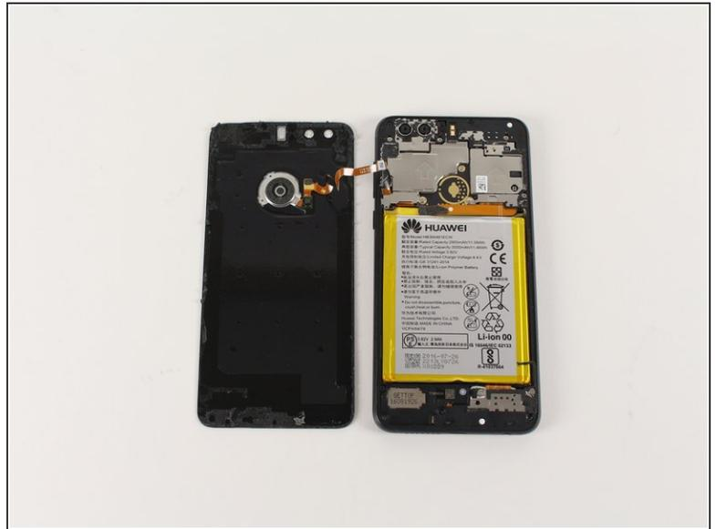
**!** Be careful not to tear the orange ribbon wire when removing the back panel.
