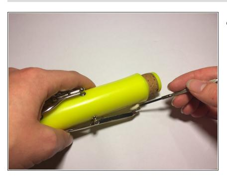
Remove the damaged pad by inserting the screwdriver under the pad and peeling it off the key.
