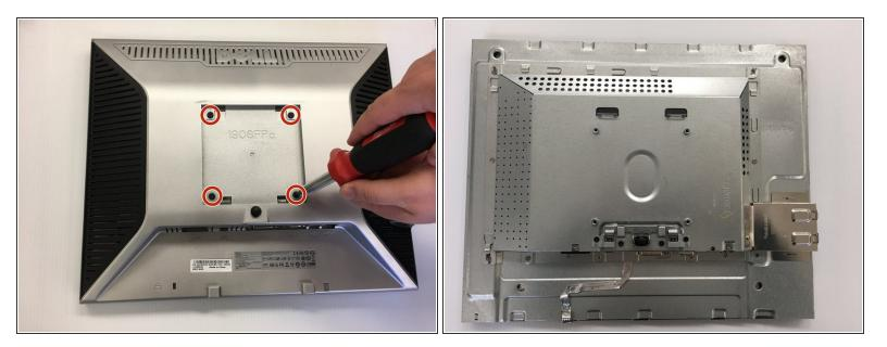
Turn the monitor over. Unscrew the four 4mm x 10mm screws on the back of the monitor and remove the plastic backing.
