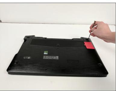
Unscrew all nine of the backplate screws with a #0 Phillips screwdriver.
