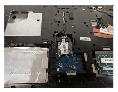
Slide the network card out of the connector.
