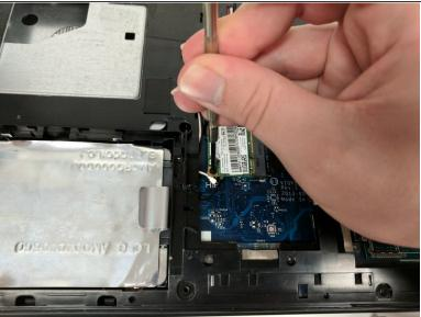
Unscrew the screw holding the network card in place with a #0 Phillips screwdriver
