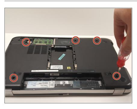
Remove the 5 bottom base screws using the 2.0mm phillips head screwdriver.
