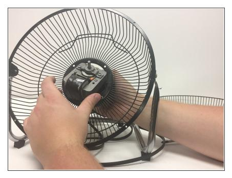
Carefully pass the motor through the opening at the back of the cage.
