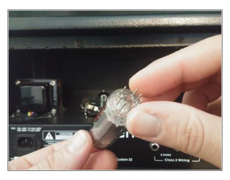
Line up the pins on the bottom of the tubes with the sockets in the amplifier.
