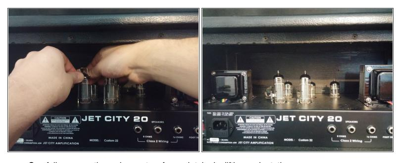
Carefully remove the spring system for each tube by lifting and rotating.
