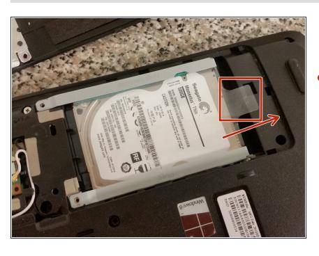
With the laptop's battery side facing you, pull the hard drive caddy's tab to the right.
