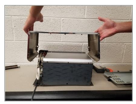
Grip the sides of the metal cover and lift the cover up off the toaster oven top.
