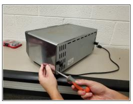
Remove the two 4mm by 8mm screws from the back of the toaster oven.
