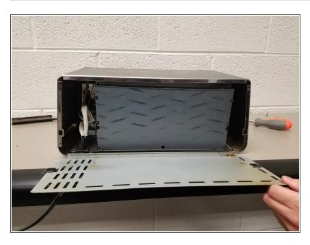
Slide the back panel off of the oven.
