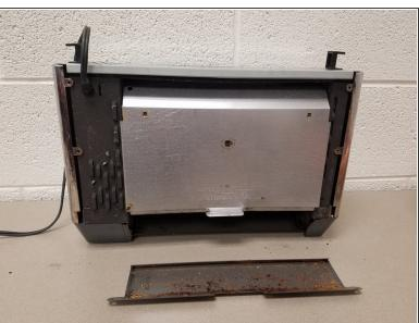
Remove the two 4mm by 4mm screws from the base in order to remove the tray.
