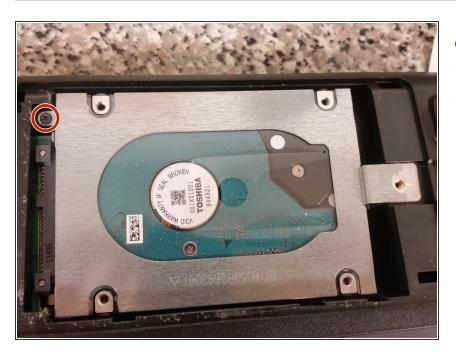
Remove the single screw securing the hard drive caddy to the base.
