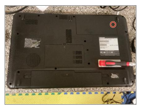
Remove the single screw securing the hard drive cover to the base.
