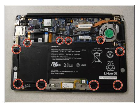
Remove the screws in the circled areas using the J0 Screwdriver to release the battery.
