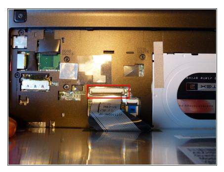
Now open the brown connector so the flat cable is loose. Then you can remove the keyboard.
