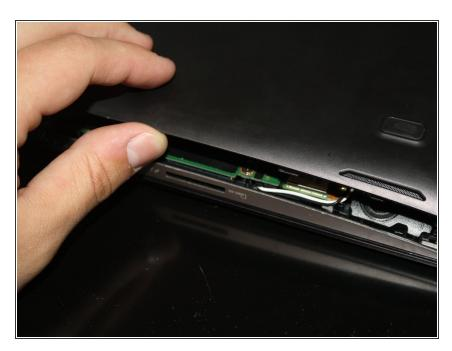
Use a plastic opening tool to open the components of the laptop. In order to do this, insert the plastic opening tool in between the two covers then pry open with your fingers
