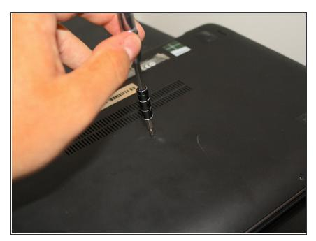
Remove the 9 1.2mm phillips head screws off the back of the computer using the small phillips head screw driver. Start by disconnecting the battery cable/ribbon.
