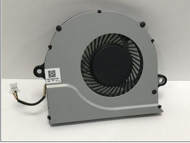
Disconnect the fan from the laptop by carefully unplugging the wires connecting the fan to the computer. The fan should now be completely detached from the computer.
