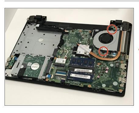
Using a screwdriver, remove the two M2.5X8 mm screws holding the fan in its place. The screws are located
