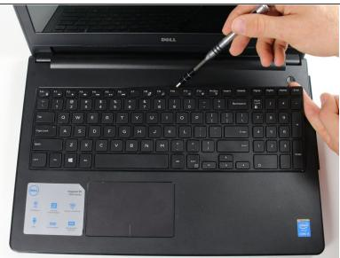
With the laptop open and facing upright, use the Spudger to pull at the notches shown in the image.
