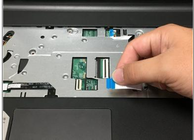
With the laptop facing upright - remove the ribbon cable from the optical drive by lifting the white release tab and gently pulling the cable away from the socket.
