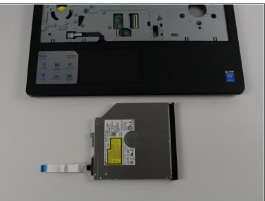
Slide the optical drive out of the port on the right-side of the laptop.
