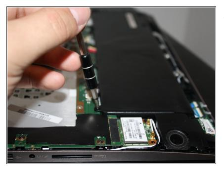
Once the back is off the device, unscrew the 7 1.2mm phillips head screws that hold the battery in place using a small phillips head screw driver
