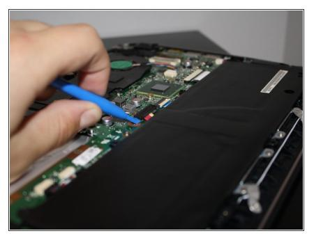
Once the screws holding the battery are out, use the plastic opening tool to disconnect the battery cable ribbon from the motherboard
