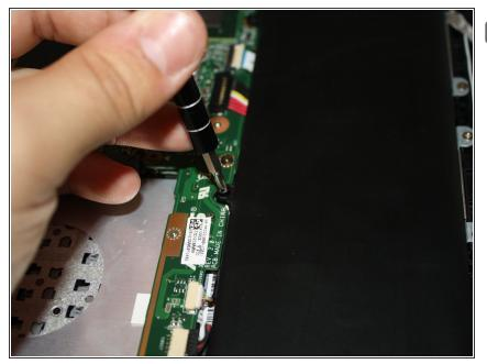
After replacing the battery, attach the wire ribbon to the motherboard and screw the designated screws back into the battery to secure it
