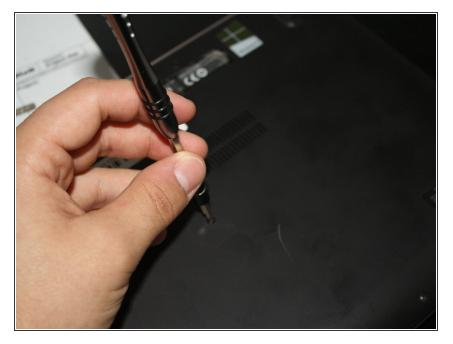
Remove the 9 1.2mm phillips head screws on the bottom of the computer using a small Phillips head screw driver.
