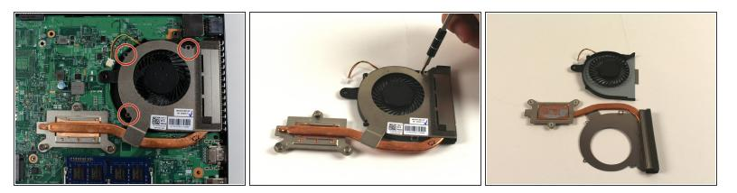
Unfasten the screws shown in the image to remove the cover and heatsink from the fan unit.
