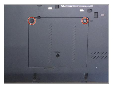
Undo the two screws that are circled, then, pry the RAM cover off by placing your finger nail or a
