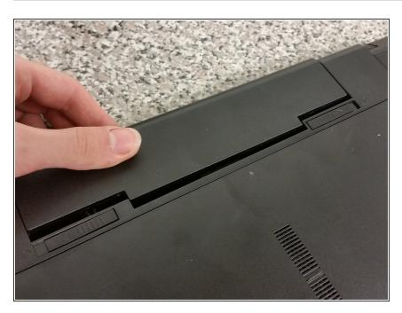
At least this part is easy. Simply push both tabs outwards, away from the center of the laptop, let go, and push/pull the battery out.
