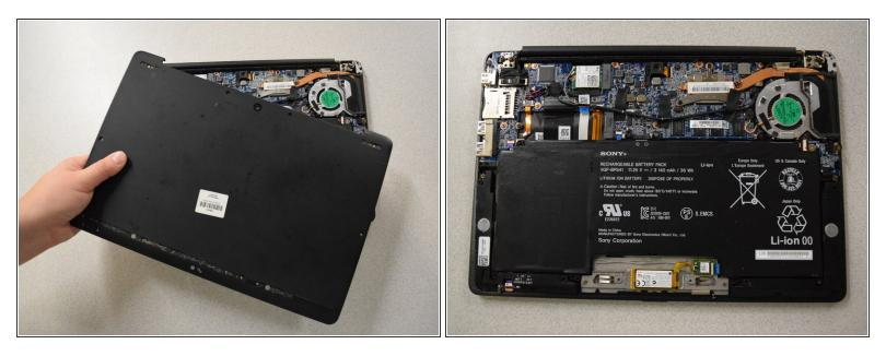
• Lift up the back cover to access internal components of the laptop.
