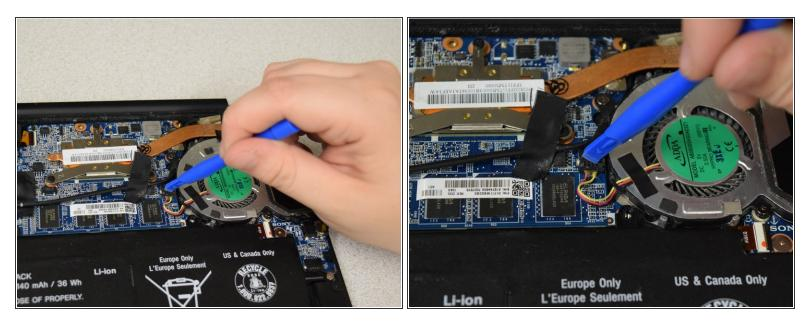
• With the aid of a the opening tool, carefully unplug the fan connector.
