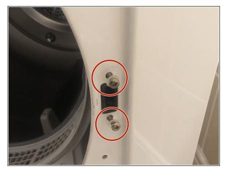
Close the front of the machine slightly and fully release the screws.
