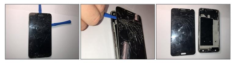
• Insert the pry tool along the side of the device, then work your way around the borders of the screen, separating the screen from the rear assembly frame.
