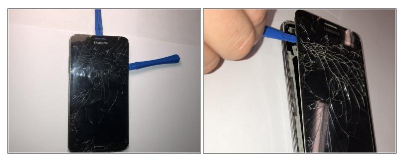
• Insert the pry tool along the side of the device, then work your way around the borders of the screen, separating the screen from the rear assembly frame.
