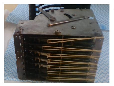
May have to slide a thin blade up the sides to break the rust free
