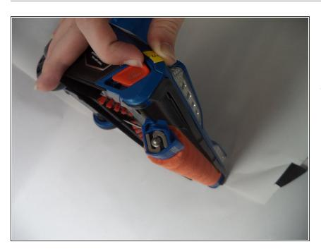
Laying the vacuum head on the its right side, push the orange "Eject Roller" switch down. The Roller can now be removed with ease.
