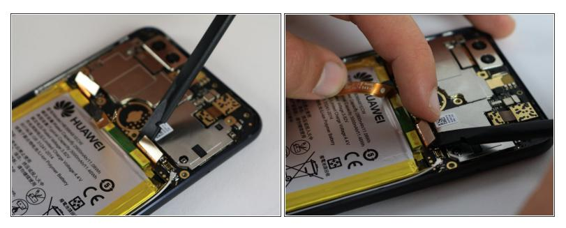
• Using a spudger, gently pry up the small connection that holds the motherboard in place.
