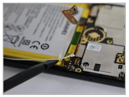
• Use a spudger to gently pry off the small antenna cable on the right side of the motherboard.
