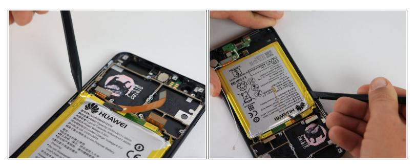
$\bigwedge$  Avoid using a heat gun for this step as overheating the battery can cause permanent damage.
