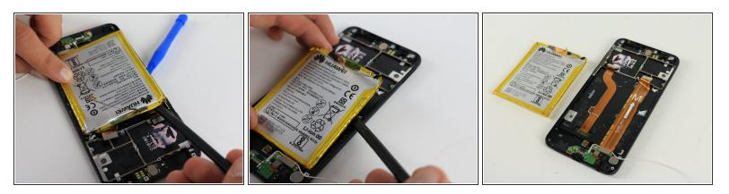
Once all the adhesive has been removed from the battery, use the spudger and plastic opening tools to gently pry the battery away from the frame.
