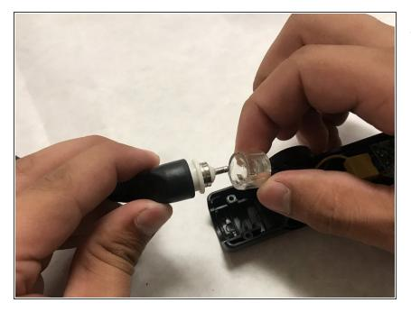
Gently pull upwards on the connection point and disconnect the power cord.
