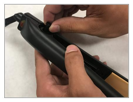
• Remove the hinge pin.
