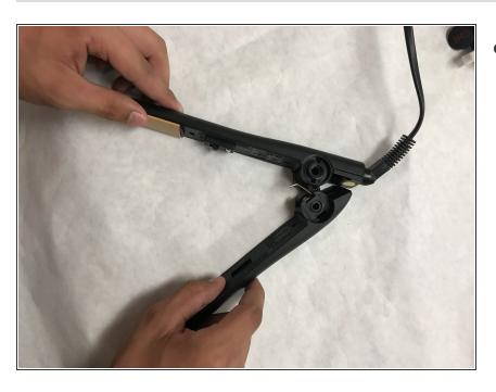
Separate the two halves of the CHI Original.
