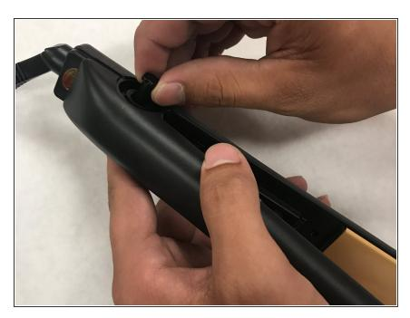
Remove the hinge pin.
