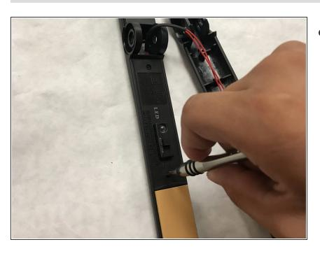
Remove the .53" long screw from the hinge pin.
