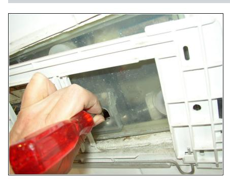
When reassembling you have to make sure that the release lever engages correctly again. Use a screwdriver if necessary. Repeat the steps in reverse order to reassemble your device.
