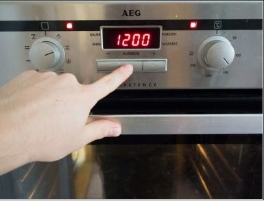
(i) If the heating and the light don't work after reassembling the oven, press a button or re-set the clock to its actual time. The heating should immediately start then.
